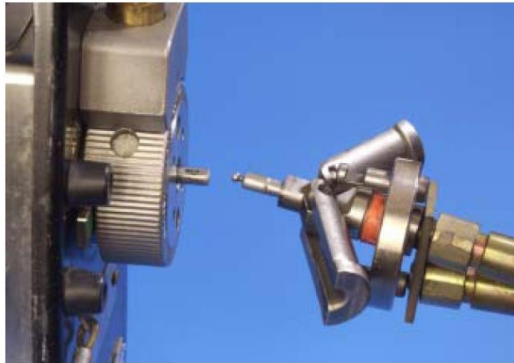
FIG. 4. Male connector on the drive cable (on the right) and female connector on the source pigtail.
