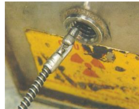
Photo 2. Source pigtail connected to drive cable.
