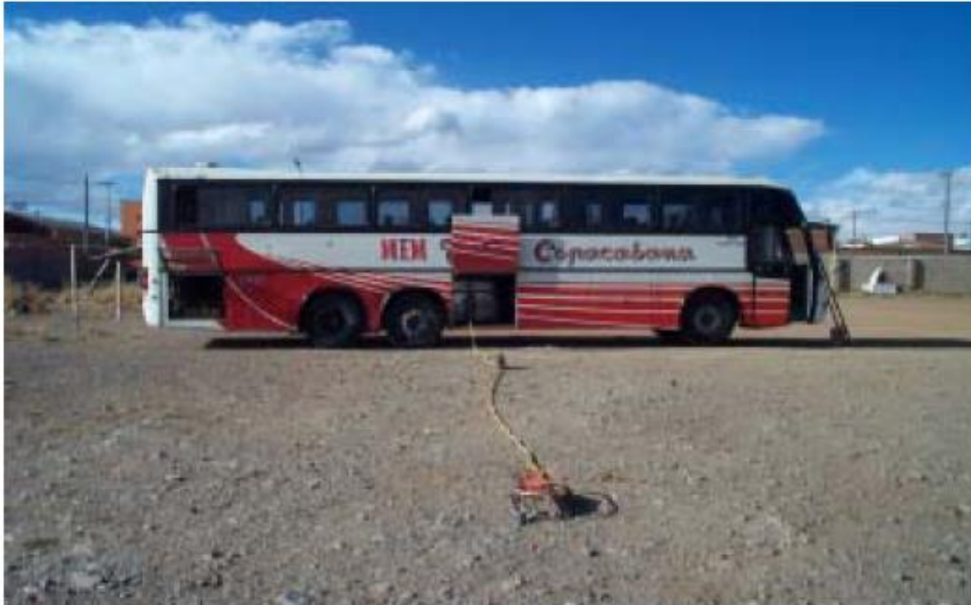
FIG. 18. Reconstruction by the IAEA of the circumstances of the accident. In the foreground is the radiography equipment with its guide tube unwound up to the cargo compartment of the bus.
